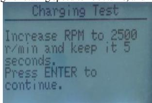
Tester starts the charging volt test after increase rev detected.
