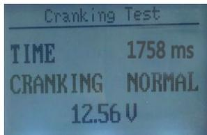
When cranking test is abnormal, battery test result will also be displayed at the same time.
