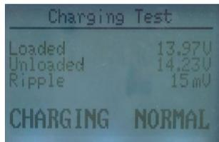
NOTE: If no increase rev detected, it shall be the fault of generator regulator or connection with battery failed. Tester will try 3 times to further detect, if still failed, it will skip the increase rev detect and the test result displays "No Volt Output".
