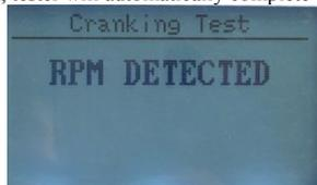
Normally, cranking voltage value lower than 9.6V is regarded as abnormal and it is OK if it is higher than 9.6V. Test result of the tester includes actual cranking voltage and actual cranking time.
