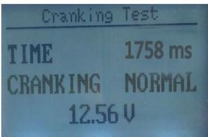
When cranking test is abnormal, battery test result will also be displayed at the same time.
