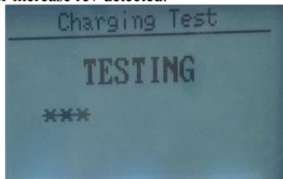
After the test finished, tester displays the effective charging volts, ripple test result and charging test result.
