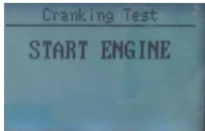
Starting the engine as prompted, tester will automatically complete the cranking test and display the result.
